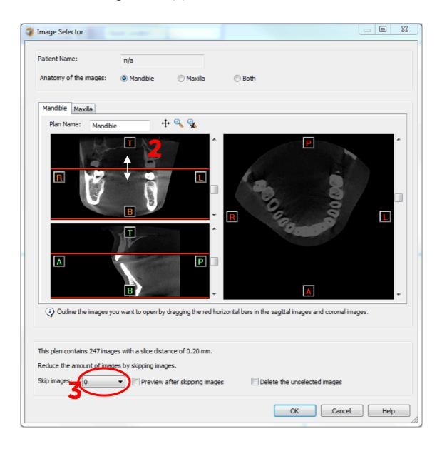
In order to further reduce software load, you can remove axial images by selecting the skipped image count different from 0 (for example: skip images = 1 selects every second image, skip images = 2 selects every 3<sup>rd</sup> image) (3). For exported DICOM image sets with a slice distance below 0.4mm, it is recommended to skip 1 image.
