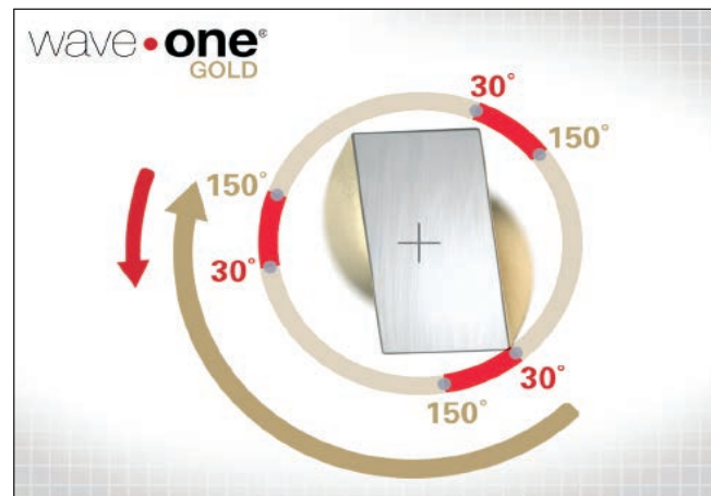
Figure 6. The WaveOne Gold files utilize unequal bidirectional angles to improve inward movement, cutting efficiency, and hauling debris out of the canal.
