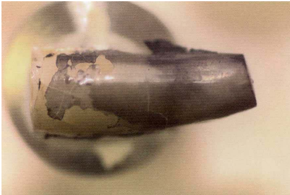
Figure 14: Dentine surface treated with Seal&Protect (two coats) after 20,000 strokes (equals 1 year) in a tooth brush abrasion test. Most areas are still covered with sealant coat (dark areas). Photo: B Schemehorn.
