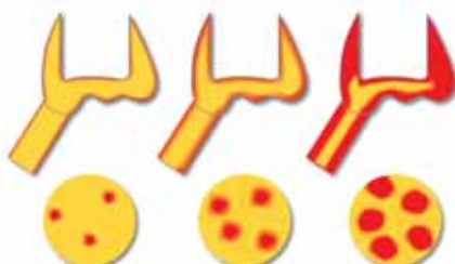
Example: Solidification sequence in a single crown
