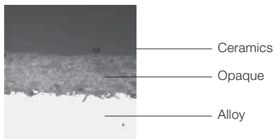
Optimized bond – Degunorm supra/Duceragold
