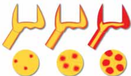
Example: Solidification sequence in a single crown
