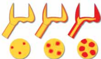
Example: Solidification sequence in a single crown
