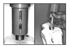
Press down on the unit's rocker switch to inject. Ensure that the mold is completely filled by viewing the blue Cartridge Plug through the Sleeve slots until the Plug stops moving.
