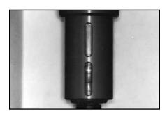
Place the Flask in the Injection Unit, ensuring that the bolts and Flask Brackets face to the operator's right side. Position the open slots on the Cartridge Sleeve facing out; then push the sleeve up toward the unit's cross head, securing the Sleeve around the blue rubber "O" ring. Gently tighten the unit Hand Wheel to secure the Flask. The Flask should be aligned completely vertical with the Injection Piston.
