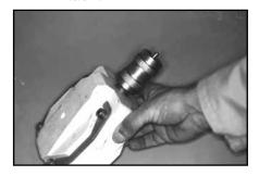
Fit the small blue plastic Piston Cap onto the end of the Pressing Device Piston.
