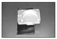
Apply petrolatum to the inside of the Microwave Flask, and place the Flask on the Leveler (side "1" up).
