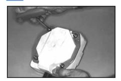
Apply separator to the DENTSPLY LabStone, and place the top half of the Flask on the bottom half, *ensuring complete, intimate contact and closure of the halves.* Secure metal Flask Brackets to the Flask and tighten using a metric wrench, specifically for the Microwave Flask.
