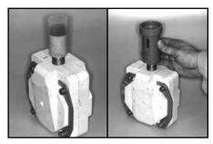
Insert the Cartridge nozzle into the plastic Injection Socket until it seats on the Injection Socket's lip. Place the metal Protective Sleeve over the Cartridge.
