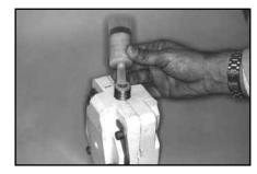
Place material into the plastic Injection Cartridge; then insert the blue plastic Cartridge Plug into the large open end, ribbed side out. Push the blue Cartridge Plug in as far as possible to compress the material.
