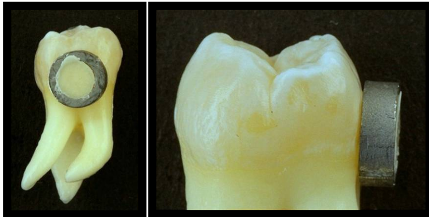
Figure 26 Glass ionomer specimen supported by a metal ring for shear bond strength testing
