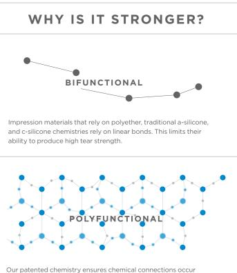
Our patented chemistry ensures chemical connections occur through polyfunctional bonds, or branching. This allows the material to be strong even at the thinnest cross-sections.
