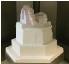
Figure 5 Placement of bridges with sintering bar (more than 9 units).
