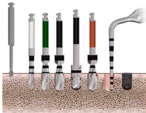
Rosenbohrer (Guide Drill) Spiralbohrer (Twist Drill 2.0) Spiralbohrer (Twist Drill 3.2) Spiralbohrer (Twist Drill 3.7) Kortikalisbohrer (Cortical Drill 3.7/4.0) Spiralbohrer (Twist Drill 3.85) OsseoSpeed® TX 4,0 S 6 mm
