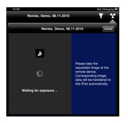
After selecting the requested image type a corresponding exposure readiness request will be sent to the remote Sidexis iX server. The server orders a new exposure readiness from Sidexis. The Sidexis iX app shows a exposure readiness dialog while waiting for the results.
