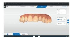
2 Export a Dentsply Sirona scan or Import an STL scan to OraCheck. One scan is used as reference scan and the 2<sup>nd</sup> one to compare.
