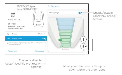
() The SHAPING TARGET Setting is OFF by default, and only available when the Propex IQ<sup>®</sup> Apex Locator is connected to the Endo IQ<sup>®</sup> App.
