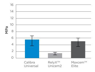
Test: Shear Bond Strength to dentin after self-curing for 6 minutes at 37°C. Source: Dentsply Sirona.
