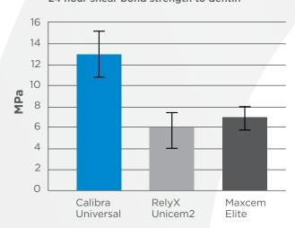
Test: Shear Bond Strength to dentin after self-curing for 24 hours at 37°C. Source: Dentsply Sirona.
