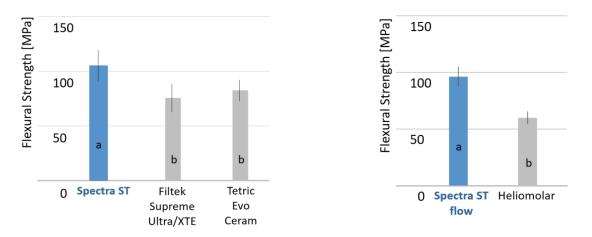
Fig. 1 Flexural strength of Spectra ST (left; Belli & Lohbauer 2015) and Spectra ST flow (right; Belli & Lohbauer 2018) in four-point bending after two weeks of water storage. Different letters indicate significant differences.
