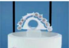
Correct position on the sintering tray
