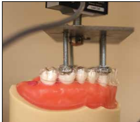
Fig. 2 Pull-off direction on Universal Testing Machine.##
