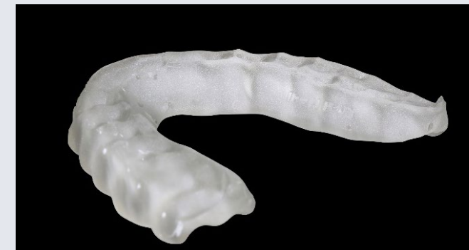
Fig 11: The 3D-printed splint after removal of the supports, cleaned and cured as a medical device for use
