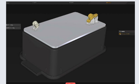
Fig 15: Preparation of the print job of the insertion tool and a temporary crown (copy of the final crown from Fig. 13) in inLab CAM 22
