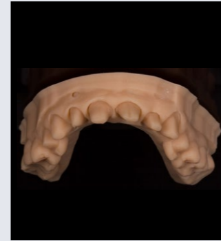
Fig 11: 3D-printed model with dies with Primeprint Model material
