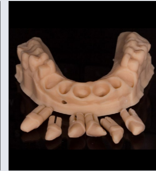
Fig 11: 3D-printed model with dies with Primeprint Model material
