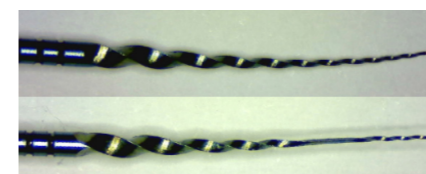
Figure 7: Plastic deformation of EdgeTaper Platinum® instrument. On the top: before shaping (no deformation). On the bottom: after shaping one canal, plastic deformation is observed.
