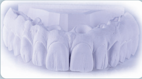
1. APPROVED PROTOTYPE DESIGN MILLED IN MONOLITHIC ZIRCONIA - ALL CONTOURING MADE IN GREEN-STAGE
