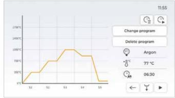
Process view with the possibility of activating predrying, adjusting process parameters, programming Auto-Start functions and displaying production time.
