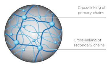
Homogenous three-dimensional structure and cross-linking of primary and secondary molecular chains
