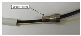
2. Feed the drive air and strain relief cord through collector body (exhaust port of collector body faces away from exterior sheath)
