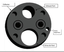
3. Slide collector body up along tubes and into collector housing. Tie a knot in the strain relief cord at the collector body to hold exhaust collector in place.
