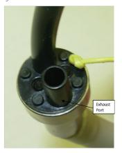
4. Attach drain tube to exhaust port on collector body and attach exhaust tube to dental unit oil connection device.
