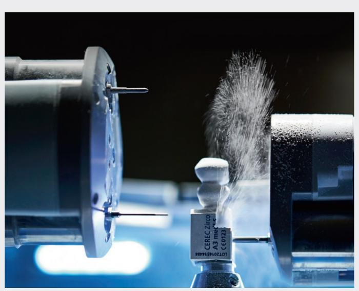
The CEREC MC XL mills a restoration with utmost precision from a block of zirconia
