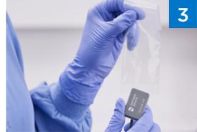
Securely hold the sensor so that it does not fall to the floor, and then discard the used cover.
