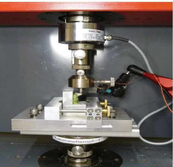
Figure 8: Fracture test set-up
